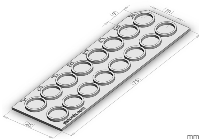
Fig. 1. Isometric schematic of 16-well nylon-based plastic slide.
